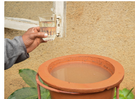
The system uses handmade ceramic filters to remove sediment and bacteria from local drinking water.
